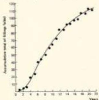
FIG. 1.—The progressive failure of 112 of the original 145 amalgam fillings over a period of 21 years. (A. D. Robinson, 1971, *Brit. dent. J.*, 130, 207).
